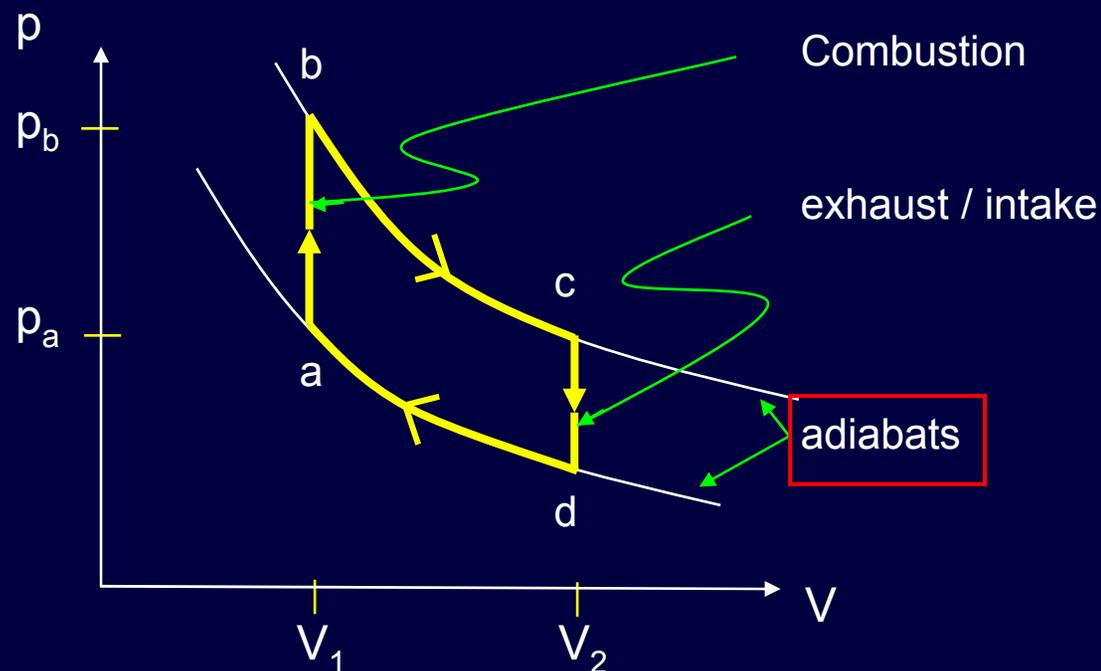
$b \rightarrow c$  and  $d \rightarrow a$  are nearly adiabatic processes, because the pistons move too quickly for much heat to flow.
