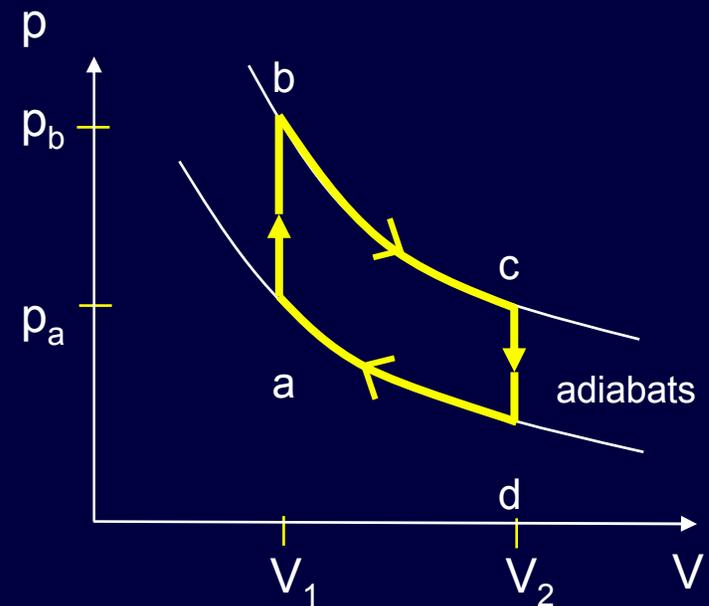
Compression ratio  $\equiv V_2/V_1 \approx 10$
