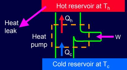
Suppose that the heat flow out of your 20° C home in the winter is 7 kW. If the temperature outside is -15° C, how much power would an ideal heat pump require to maintain a constant inside temperature?
