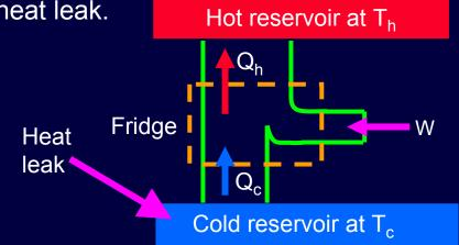
There is a 70 W heat leak (the insulation is not perfect) from a room at temperature 22° C into an ideal refrigerator. How much electrical power is needed to keep the refrigerator at -10° C? Assume Carnot performance.
