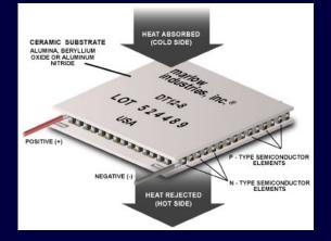
Electrons pushed from electron-deficit material (p-type) to electron-rich material (n-type); they slow down, cooling the top connector. Similarly, they heat up in going from n to p-type (bottom connector).
