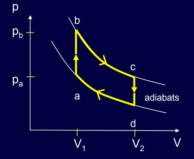
Compression ratio =  $V_2/V_1 \approx 10$  $\gamma = 1.4$  (diatomic gas)  $\rightarrow \varepsilon = 60\%$
