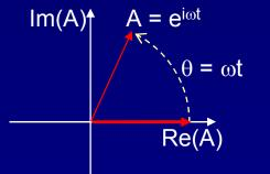
At t = 0,  $\theta = 0$ , so A = 1 (no imaginary component). As time progresses, A rotates counterclockwise with angular frequency  $\omega$ . This is the math that underlies phasors.
