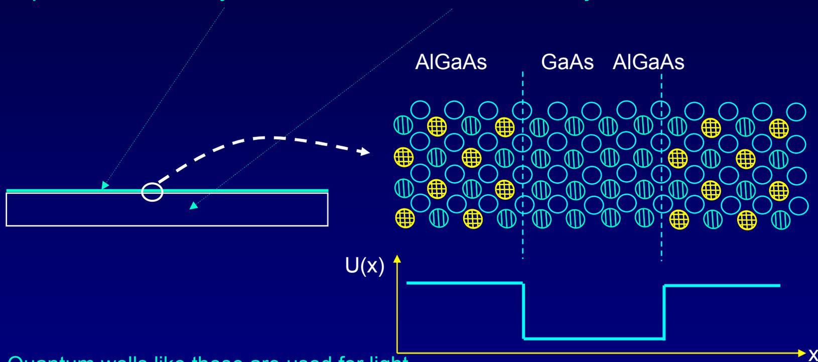
Quantum wells like these are used for light emitting diodes and laser diodes, such as the ones in your CD player.
