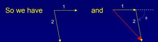
Note that the algebraic solution we wrote before does not apply here, because the amplitudes aren't equal. You can use some trigonometry to calculate the length of the third side of the triangle.
