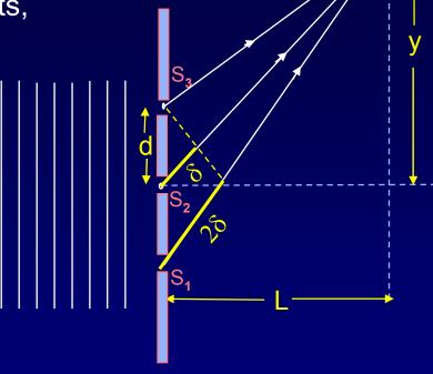
The positions of the principal interference maxima are the *same* for any number of slits!
