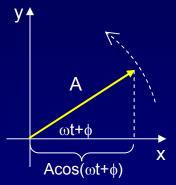
It is conventional to draw one phasor horizontal. Because the phasors are rotating, this merely means we are looking at them at a particular time.
