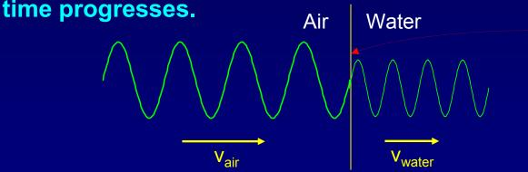
Continuity of the wave at the air-water interface (at all times) requires that the frequencies be the same.
