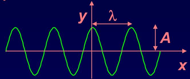
For a wave on a string, each point on the wave oscillates in the  $y$  direction with simple harmonic motion of **angular frequency**  $\omega$ .
