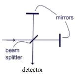
9. After painstakingly tuning your Michelson interferometer, such that there is maximal constructive interference, your lab partner bumps one of the outer mirrors, reducing the path length of that arm of the interferometer. You notice that your photometer (a tool for measuring the intensity of light) reading has not changed. What is the minimum distance that the mirror could have been bumped?
