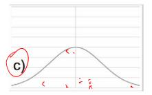
Figure c: There will no longer be interference fringes, but the overall envelope will be slightly wider.
