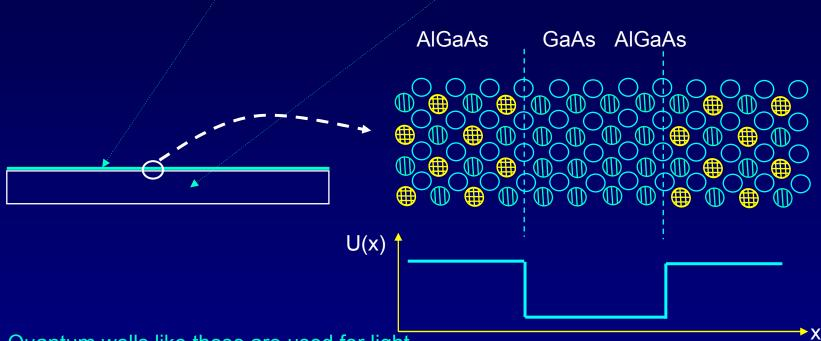
Quantum wells like these are used for light emitting diodes and laser diodes, such as the ones in your CD player.
