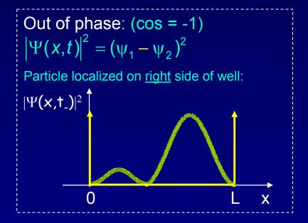
The frequency of oscillation is  $\omega = \omega_2 - \omega_1 = (E_2 - E_1)/\hbar$ , or  $f = (E_2 - E_1)/\hbar$ . This is precisely the frequency of a photon that would make a transition between the two states.
