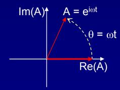
At t = 0,  $\theta = 0$ , so A = 1 (no imaginary component). As time progresses, A rotates counterclockwise with angular frequency  $\omega$ .
