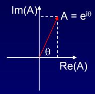
The Argand diagram of a complex number, A, puts Re(A) on the x-axis and Im(A) on the y-axis. Notice the trig relation between the x and y components.  $\theta$  is the angle of A from the real axis. In an Argand diagram,  $e^{i\theta}$  looks like a vector of length 1, and components ( $\cos\theta$ ,  $\sin\theta$ ).
