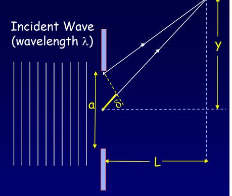
The second minimum is at an angle such that the light from the top and a point at a/4 destructively interfere:
