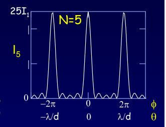
The positions of the principal maxima occur at  $\phi = 0, \pm 2\pi, \pm 4\pi, ...$  where  $\phi$  is the phase between adjacent slits.  $\theta = 0, \pm \lambda/d, \pm 2\lambda/d, ...$
