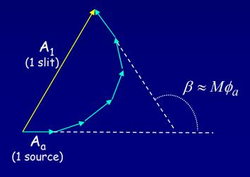
Destructive interference occurs when the polygon is closed ( $\beta = 2\pi$ ):
