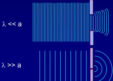
The transmitted wave is concentrated in the forward direction, and at near distances the wave fronts have the shape of the aperture. The wave eventually spreads out.
