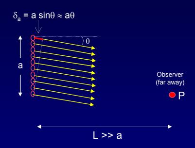
$\beta$  = phase difference between waves coming from the top and bottom of the slit.
