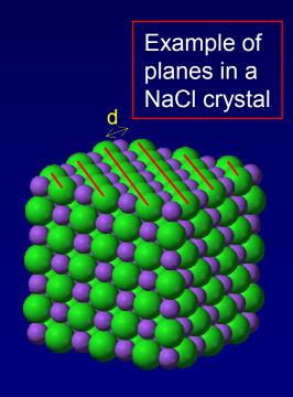
Each crystal has many values of d - the distances between different planes. For a known wavelength  $\lambda$  the observed angles  $\theta$  can be used to determine the crystal structure.
