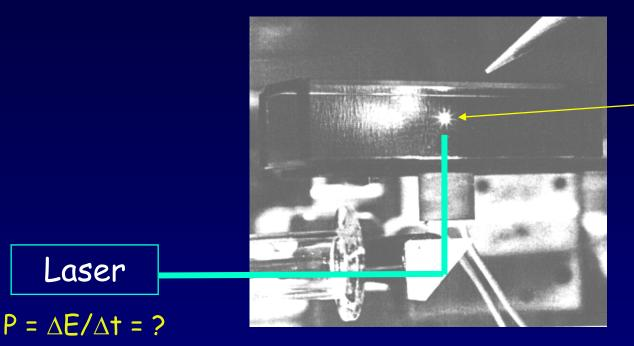
Glass bead 'floating' on a laser beam! (AT&T Bell Labs)
