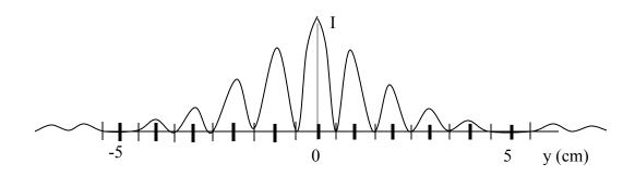
As in our laboratory experiment, the following interference pattern is observed on a screen located 2 m from slits illuminated by a coherent light source with the wavelength of 633 nm.
