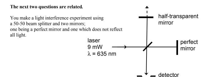
Because the top mirror is not perfectly reflective (half the light is actually transmitted), the power measured at the detector when only the vertical arm is blocked is 2.25 mW, while the power measured at the detector when only the horizontal arm is blocked is only 1.125 mW. **Assume identical length arms.**
