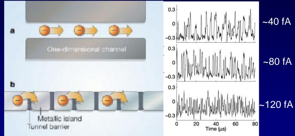
Electrons that successfully tunnel through the 50 junctions are detected using a fast single-electron transistor (SET).
