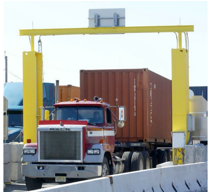
A truck passes through a radiation portal monitor at the port of Newark, New Jersey.
