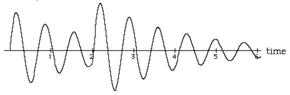
At the instants of the impulses ( t=0 and t=2), the slope changes discontinuously. Note that the above particular solution, constructed by superposition of impulse responses G, is a particular solution to
