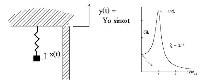
The equation of motion is, (for x defined as the absolute displacement, i.e., relative to the lab, not the ceiling) neglecting the dissipation terms,
