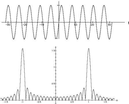
Consider an  $\infty$  cycle sine wave  $x(t) = \sin \alpha t$  for all t. In this case its FT is  $(\pi/i)[\delta(\omega+\alpha)-\delta(\omega-\alpha)]$  and has amplitude  $|\cdot|$  only at the apparent frequency. It appears that the FT requires a large amount of time duration of a sine wave before it will unambiguously single out a particular  $\omega$ .
