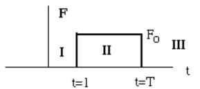
We3 will take the system to be undamped, so  $G(t) = \sin(\omega_n t)/m\omega_n$ .
