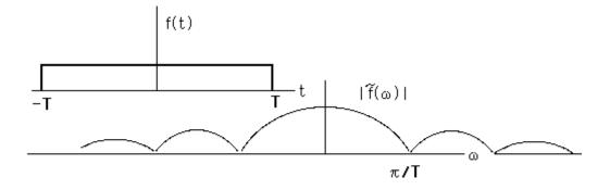
This function of frequency is peaked at zero ( with magnitude = 2T = area under the curve in the time domain ) and dies away as  $\omega$  gets to be of order  $2\pi/T$  or larger. In a plot one can
