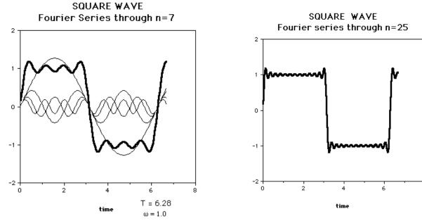
The truncated Fourier series has difficulty capturing the very fast transitions. The overshooting followed by, or preceded by, a ringdown is called the "Gibbs" phenomenon and is characteristic of a truncated Fourier series's attempt to describe sharp changes in behavior such as discontinuities.
