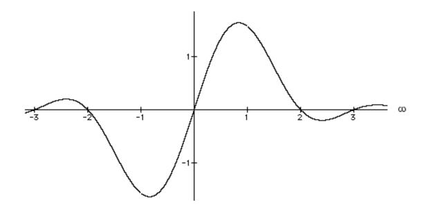
Consider a 10 cycle sine wave  $x = \sin(10 \pi t/T)$  for -T<t<T, and x=0 otherwise. Such an x(t) might be termed a "tone burst". It has a nominal frequency of 10  $\pi t/T$  and a FT of
