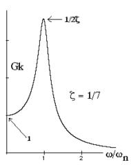
say that resonance occurs at  $\omega_n$ . At that point G is seen to be  $1/(2k\zeta)$ . This will be large if  $\zeta$  is small, and infinite when  $\zeta = 0$ .
