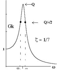
**Definition:** Quality Factor "Q" = the peak value of G compared to its quasi static value at  $\omega = 0$ , G = 1/k. The maximum amplification possible. See plot. It happens at  $\omega \sim \omega_n$ . Our theory tells us that  $Q = 1/2\zeta$ .
