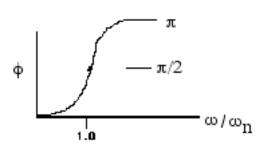
The high frequency mass controlled region is on the right and has  $\phi$  approximately equal to  $\pi$ . Thus the displacement is 180° behind the force. Note however, that the acceleration is in phase with the force, as it should be when we recall  $F(t) \sim ma$ .
