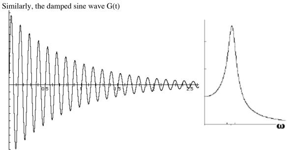
has a  $|\tilde{G}(\omega)|$  as already plotted several times.  $|\tilde{G}(\omega)|$  peaks with a finite value at the nominal frequency, but has non-zero amplitude at other frequencies too.
