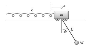
Calculate the general solution for x(t) and  $\phi(t)$ , where both variables are measured with respect to their equilibrium positions. Consider <u>small oscillations</u> only, i.e. small variations of x and  $\phi$  from their equilibrium positions.
