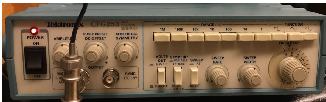
Figure 5. Tektronix Waveform Generator. [4]
