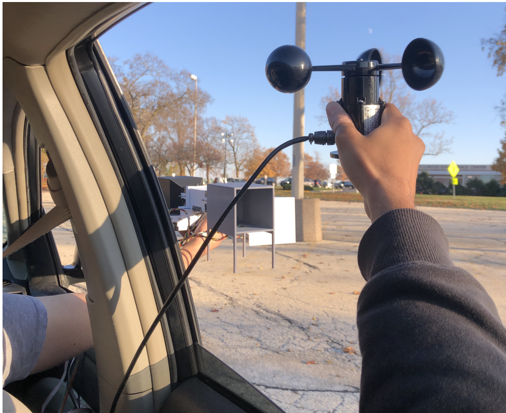
Figure 9: Experimental setup of the calibration test using a car
