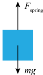
Figure 5: A model showing the force balance we used to determine the force from linear and nonlinear rubber bands.
