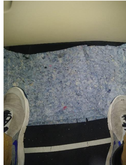
Figure 3: Insulation placement for Experiment 2 in passenger's footwell. This is a quadruple layer of 0.25" thick recycled denim sound absorber, making our layer about 1" thick, our layer is 29" wide and is 12" long.
