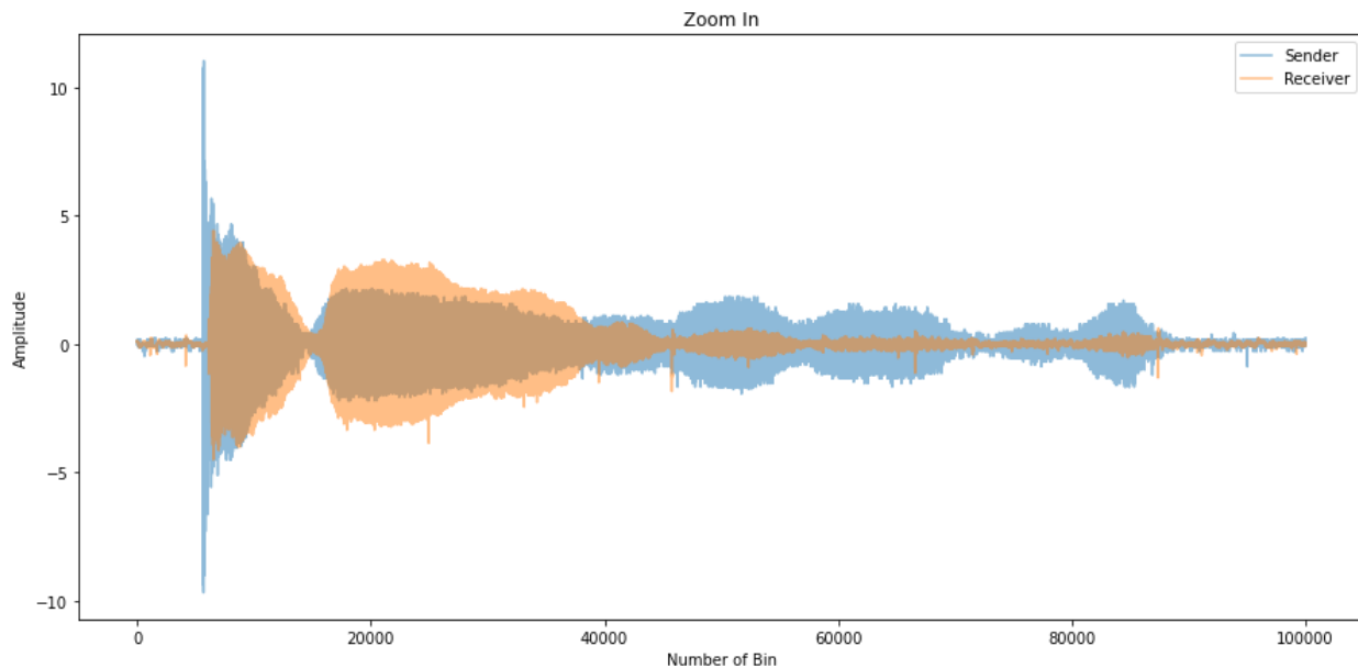
Fig 31: Comparing the zoomed in signal patterns (after cropping) between the sender side (blue) and the receiver side (orange). Both envelopes are cropped, the sender's envelope shown starts from bin = 45000; the receiver's envelope shown starts from bin = 55000, both have a length of 100000 bins.
