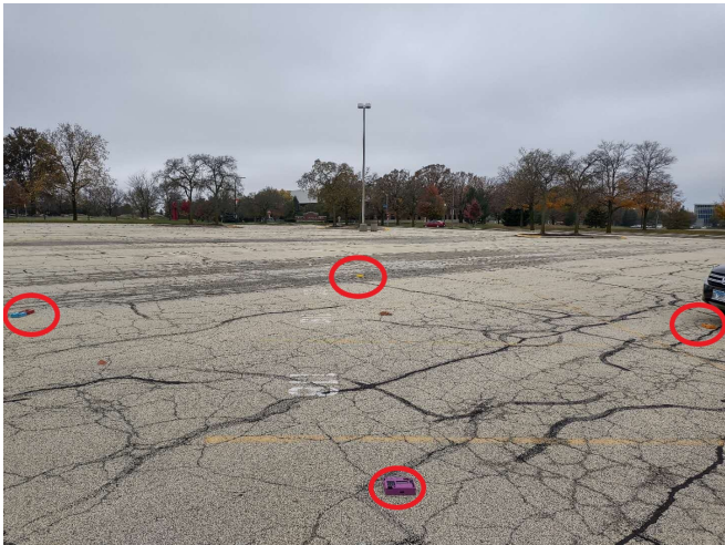
FIG. 3. Illustration of a test setup for Fig. 1 (a). Five Arduinos are put on the vertices of a diamond/square, marked in red circles. There are two Arduinos at the left vertex and the remaining three Arduinos are at the other three vertices. The car is directly at the right vertex and plays a beep sound. In our analysis, we rotate the diamond so that the car is at the top corner, but all relative positions will remain unchanged.
