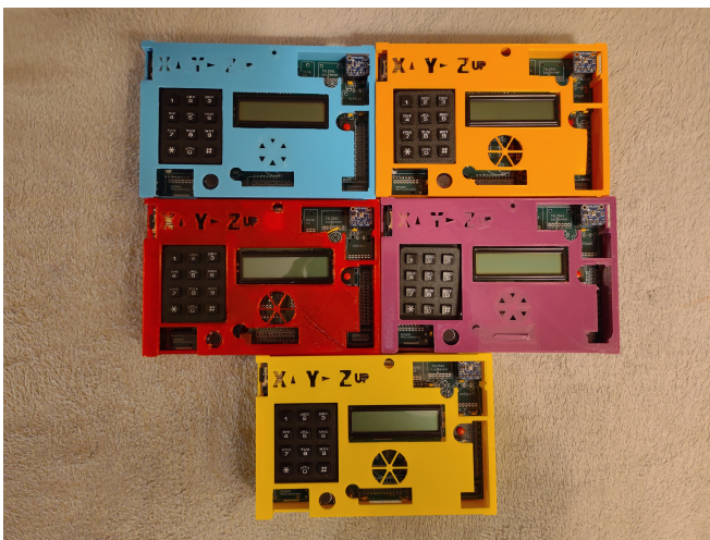
FIG. 15. Five final PCB version of the recording devices.
