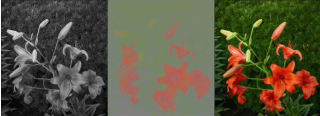
Figure 6: A comparison of the Luminance and Chrominance of a given color image, demonstrating how they combine.
