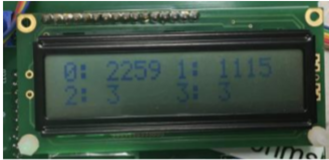
Figure 19: LCD attached to the PCB. The LCD is displaying the DAC counts of the four LEDs: red (0), green (1), blue (2), and yellow (3).
