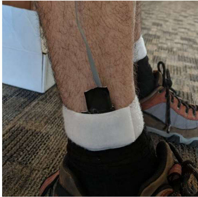
Figure 2: The accelerometer-gyroscope sensor strapped to a subject's ankle
