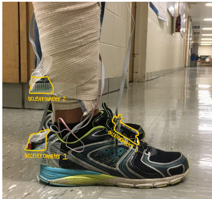
Figure 3.3: Accelerometer placement on foot and calf
