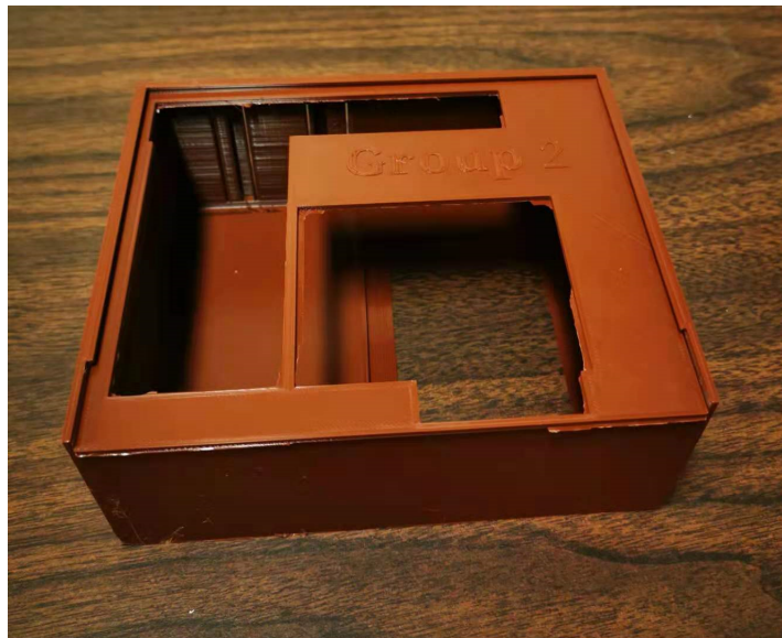
Figure 3.13: 3D-printed case for the data logger
