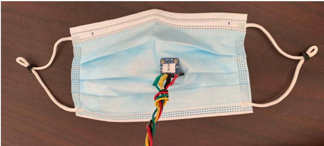
Figure 2.4: Outside of a surgical mask with the pair of BME680s attached. The “outside” BME680, labelled 0x76, is visible from the outside of the mask.
