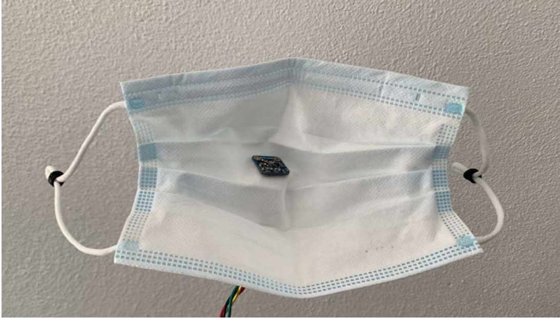
Figure 2.5: Inside of a surgical mask with the pair of BME680s attached. The “inside” BME680, labelled 0x77, is visible from the inside of the mask.
