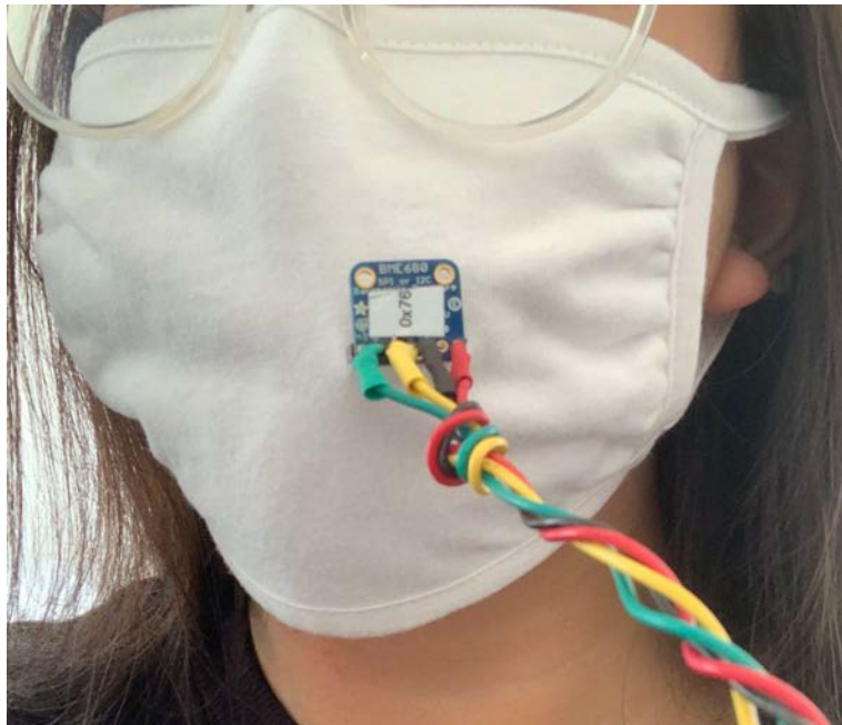
Figure 2.7: Participant wearing a white cloth mask with BME680s attached through the center of the mask.
