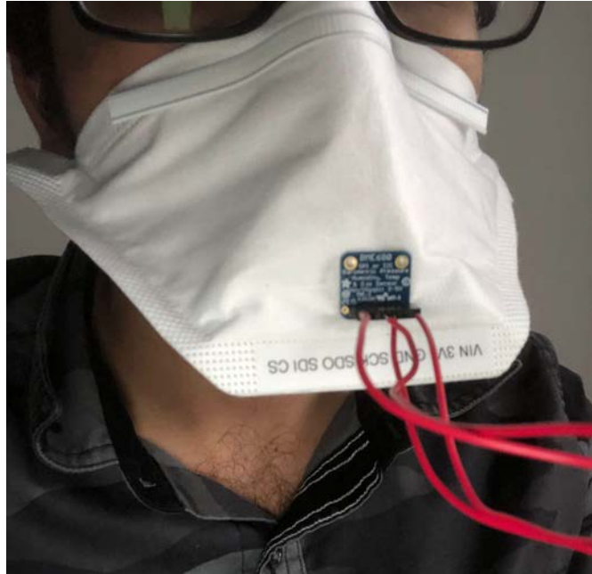
Figure 2.9: Participant wearing a N95 mask with BME680s attached through the center of the mask.
