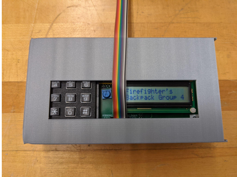
Figure 6: Backpack processor board in the 3D printed case
