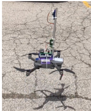
Figure #2: DJI Mavic 2 Pro with all the measuring equipment assembled taking off from the ground
