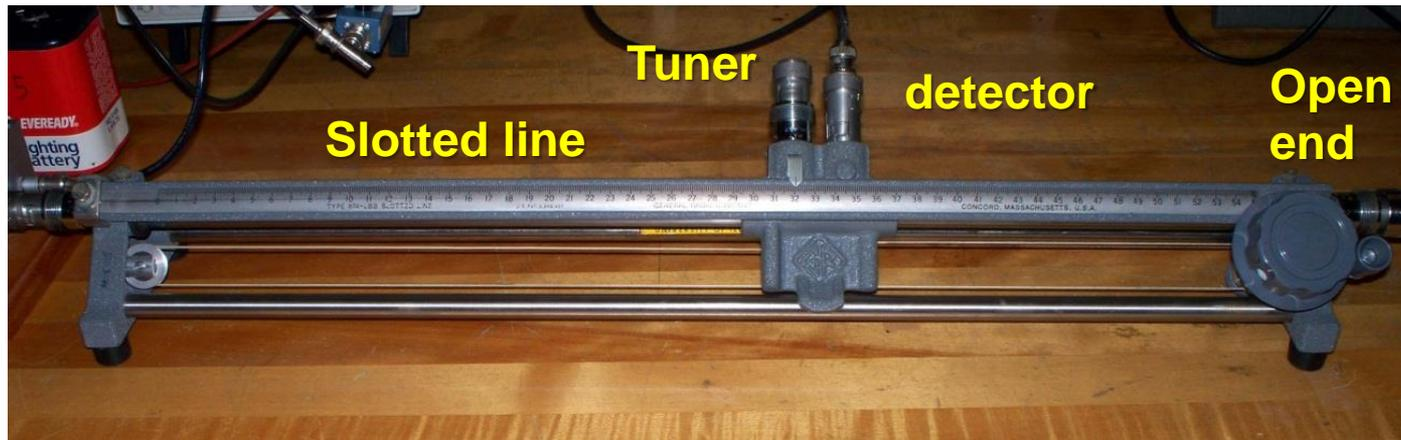
Use detector to find distance between minimums in the slotted line (wave guide)
