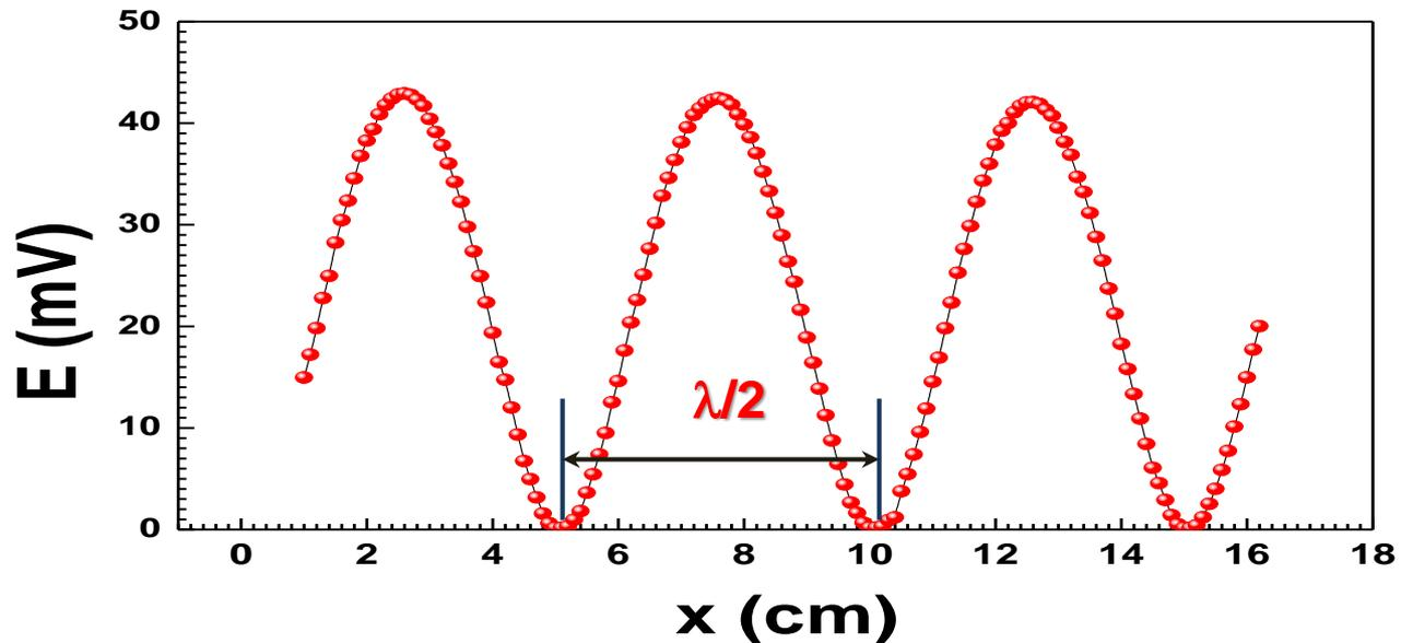
Use detector to find distance between minima in the slotted line (wave guide). Distance between consequent minima correspond  $\lambda/2$
