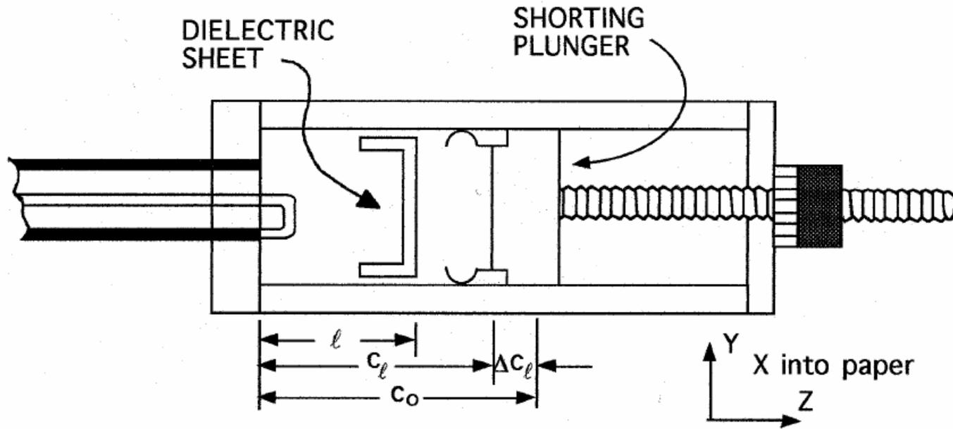
Presence of dielectric reduces length of cavity at a given resonance frequency  $\omega_0$ .
