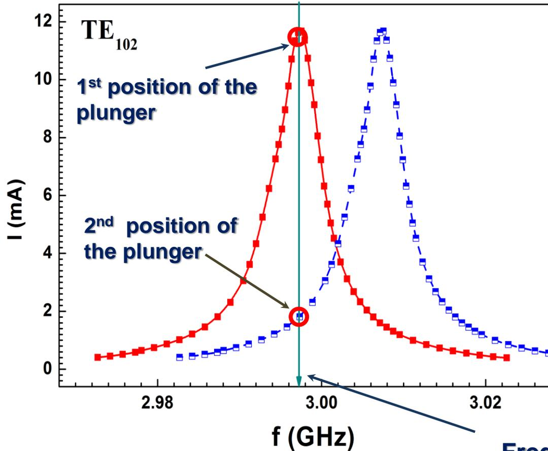
By moving the plunger we changing the resonance frequency of the cavity
