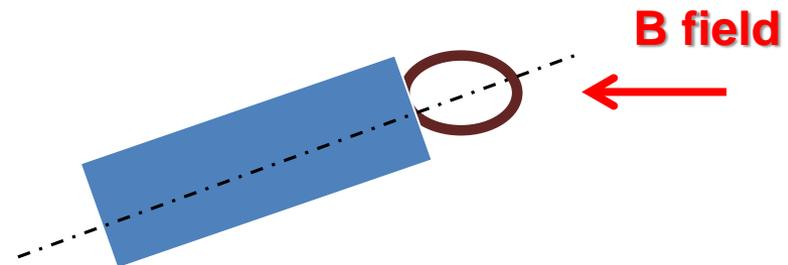
**While in resonance: turn orientation of the input loop from the vertical direction in  $10^\circ$  steps to  $360^\circ$ .
