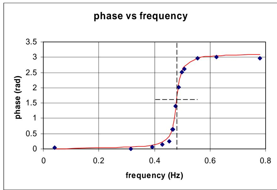
$$\omega_1 = \sqrt{\omega_o^2 - (\gamma/2)^2} \quad 3.017 \text{ rad/s}$$
