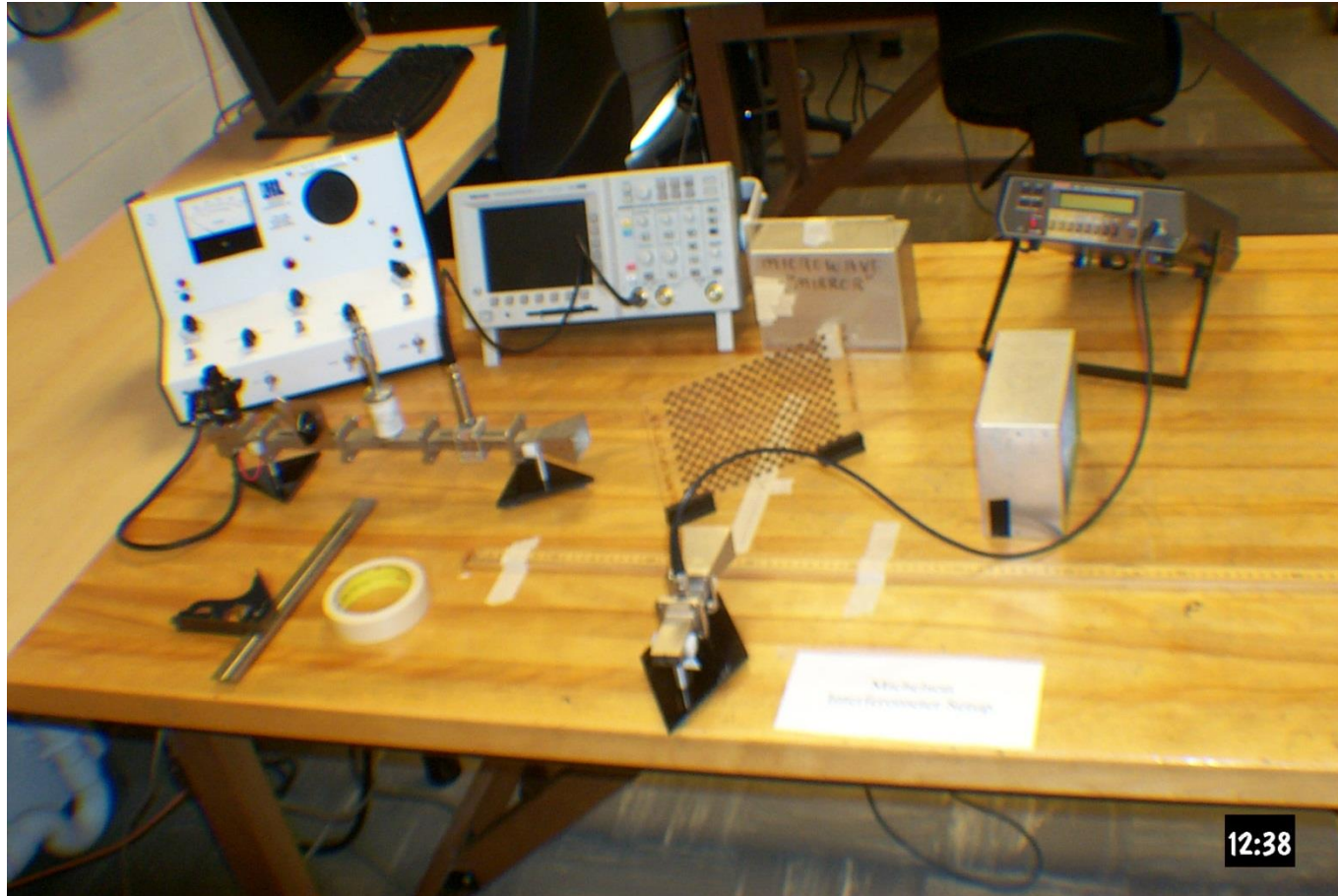
Physics 403 Lab Michelson interferometer setup
