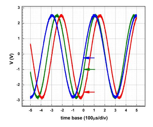
This data was taken from scope in ASCII format and plotted using Origin. Color arrows indicate the triggering levels for each trace
