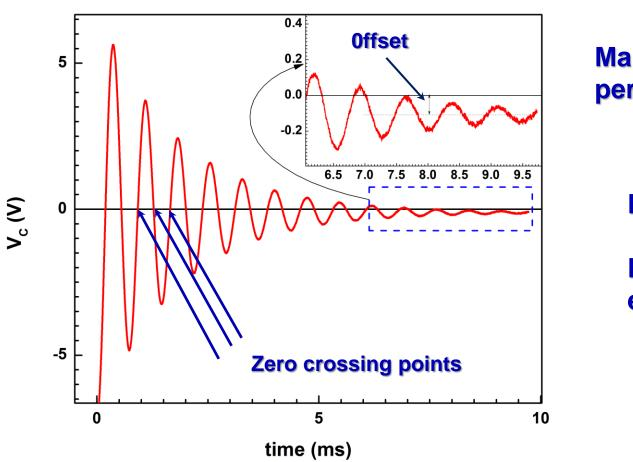
$$q(t) = Ae^{-at}sin(\omega t + \varphi) + offset$$
