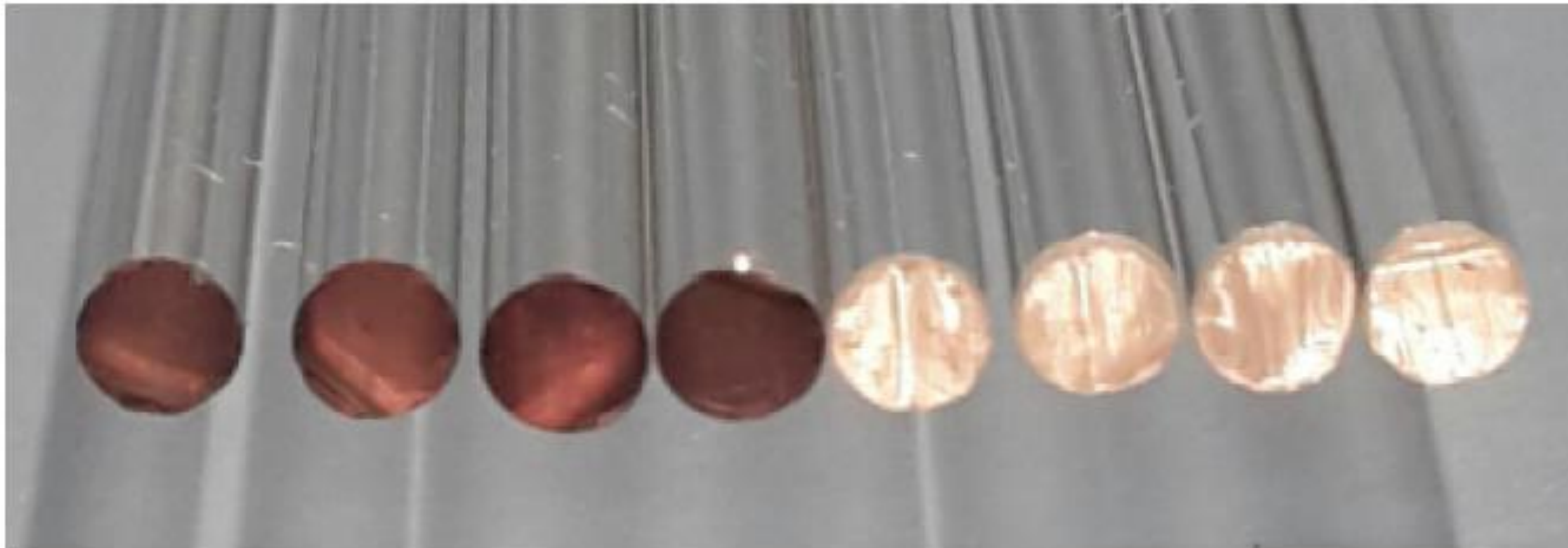
Figure 2.18: Comparison between brand new GE214 [41] fused quartz rods (right) and the same type of rods irradiated in the LHC during Run 1 ( \sim 10 MGy, left).
