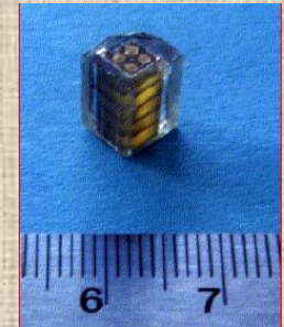
Transducer stack for ultrasonic sonar application (TRC Ceramics)
