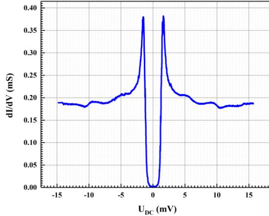
Energy gap derived from tunneling conductivity
