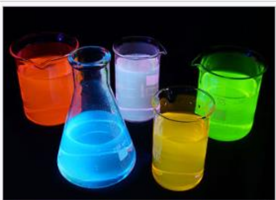
Fluorescent solutions under UV light. Absorbed photons are rapidly re-emitted under longer electromagnetic wavelengths.
