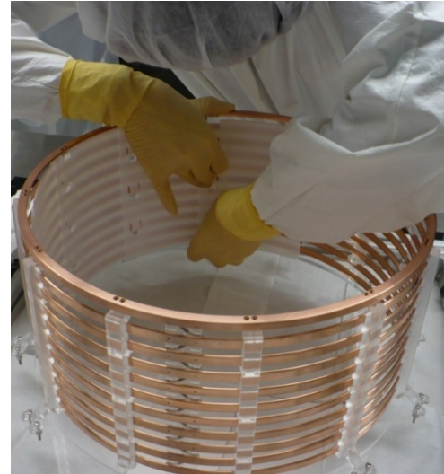
Installing field cages and teflon reflectors
