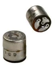
The typical mean/average sensitivity of the Knowles Acoustics omni-directional electretcondenser pressure microphone + preamp that we routinely use in the UIUC Physics of Music/Musical Instruments Lab, determined at f = 1 KHz and SPL = 94.0 dB using an EXTEC 407768 SPL meter (C-weighted) and a Fluke 77 DMM on RMS AC volts is:
