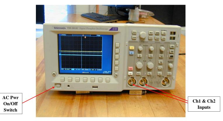
Oscilloscopes are devices used to display time-varying voltage signals. The Tek 3012 'Scope can display two such signals simultaneously (the yellow and blue traces on the above screen).
