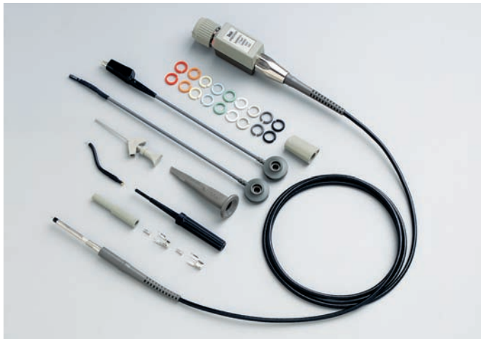
Figure 40. A typical passive probe with accessories.
