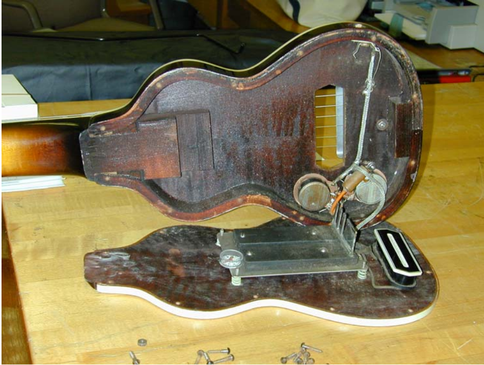
Figure 9: The Insides of a 1939 Gibson EH-150 Electric Hawaiian Guitar.
