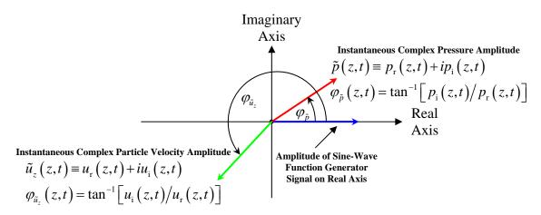
For <u>small</u> amplitudes, the instantaneous complex pressure and instantaneous 3-D complex vector particle velocity are related to each other via Euler's equation for compressible, inviscid fluid flow {inviscid fluid flow means that any/all viscous/dissipative forces  $\ll$  inertial forces}:
