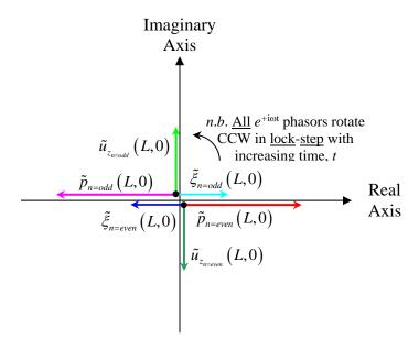
The complex <u>specific</u> longitudinal acoustic impedance at z = L on the resonances of the SWT is purely imaginary and time-independent:
