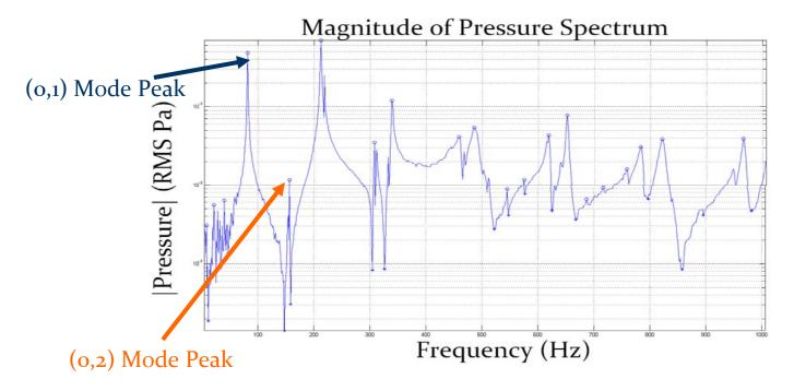
Left: A typical pressure spectrum. This scan was taken with the magnet at the center, so only (0,n) modes are accessible. The peaks correspond to eigenfrequencies of the drumhead.
