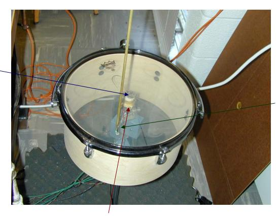
3) Once the drumhead is vibrating on a resonant eigenfrequency, the p/u microphones can be scanned over the drumhead
