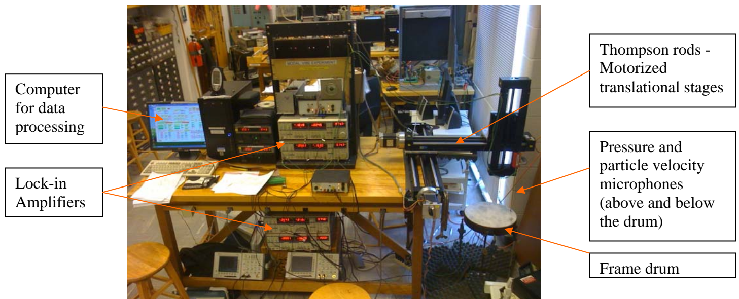
Fig.3: Picture taken inside the lab showing the DAQ system for acoustic holography.
