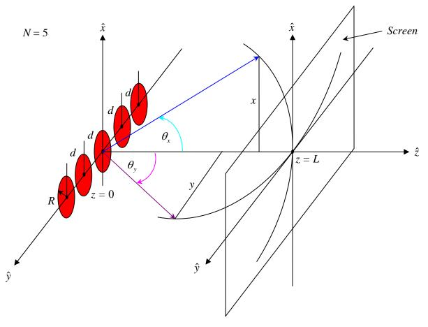
The expression for interference-diffraction associated with a 1-D linear array of N circular aperture is given by the product of interference × diffraction factors:
