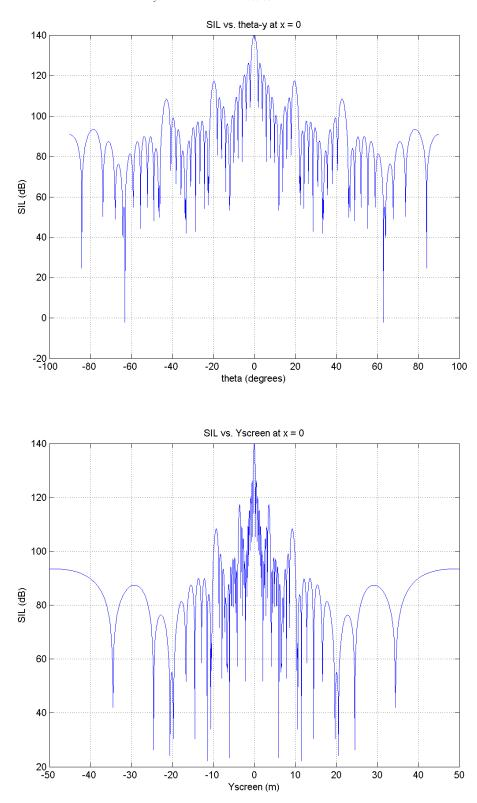
Plots of *SIL vs.*  $\theta_y$  and *SIL vs.*  $y_{screen}$  for N = 10, R = d = 1.0 m:
