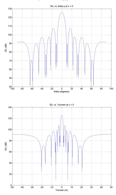
Plots of SIL vs.  $\theta_y$  and SIL vs.  $y_{screen}$  for N = 2, R = d = 1.0 m:
