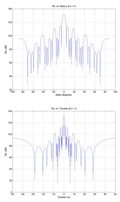
Plots of *SIL* vs.  $\theta_y$  and *SIL* vs.  $y_{screen}$  for N = 4, R = d = 1.0 m:
