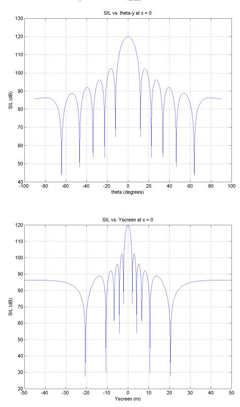
Plots of SIL vs.  $\theta_y$  and SIL vs.  $y_{screen}$  for N = 1, R = d = 1.0 m:
