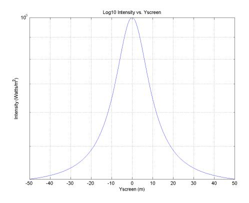
Plots of SIL vs.  $\theta$  and SIL vs.  $y_{screen}$  for R = 0.1 m:
