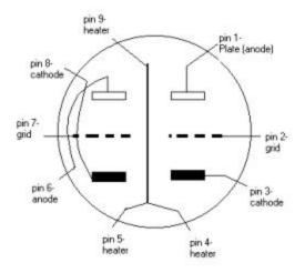
The actual tubes contain cylindrical cathodes with the filament inside of it. The control grid is a coil of wire on top of the cathode, and the cathode with the grid is placed inside another cylinder, which serves as the anode.
