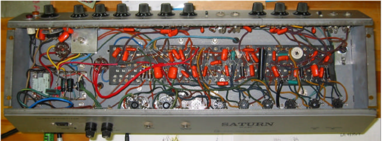
Figure 7 – Amp Chassis before removing Twin-T filters and replacing capacitors
